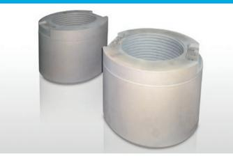
Surface treatment for the prevention of wear and seizure of copper alloy parts. This treatment is obtained by tin base electrolytic plating followed by diffusion heat treatment at 400°C (752° F).
